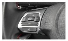
Connecting the multifunction steering wheel The IR-IN input can be used to connect optionally available CAN/Stalk interfaces, connecting the Z-N976 to the vehicle CAN and the buttons of the multifunction steering wheel.
