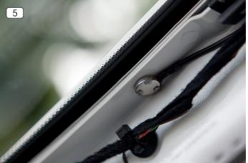
5. Take the magnetic earthing strap and attach it onto the A-pillar (metal part).
