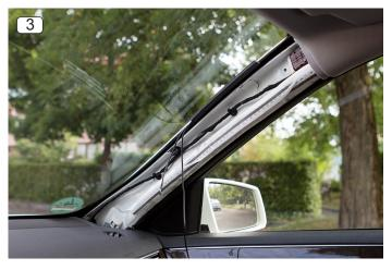
3. Remove the protective film from the window mount antenna (No. 1) and attach it so it is flush with the ceramic line.
