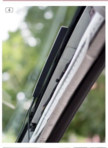
4. Carefully rub the window mount antenna (No. 1) onto the windscreen to ensure that it is affixed securely.
