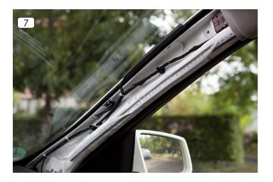
7. Use cable ties to attach the antenna cable to the existing wiring harnesses in the vehicle.
