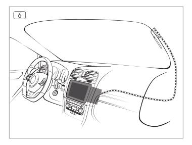
6. Route the antenna cable downwards along the A-pillar, along the dashboard and into the radio bay.
