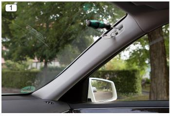
Remove the A-pillar cover in your vehicle. The cover is secured with special clips.
