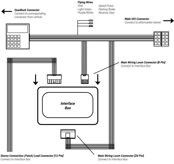
Note: Must be connected first, before power connection is made to the interface
