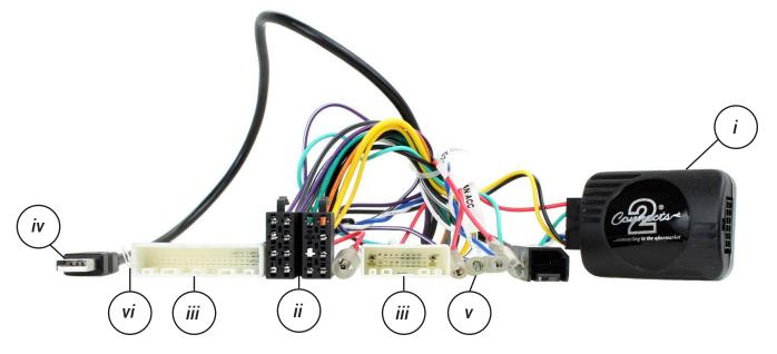
i. Interface Box ii. Female ISO Connector iii. Vehicle Specific Connector (40 Pin/20 Pin) v. Flying Wires (Park Brake, Rev Gear, ACC 12V) vi. 5mm Ground Terminal
