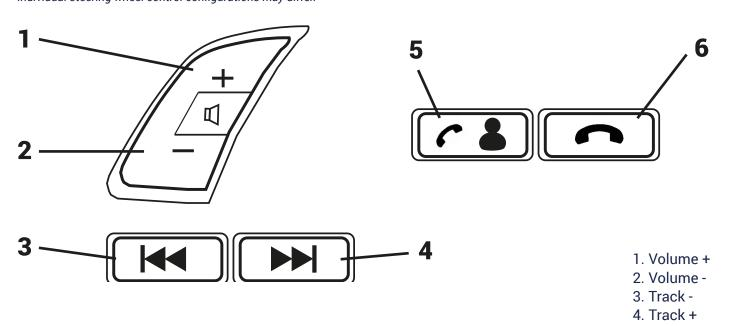
5. Pick Up 6. Hang Up Before installing the interface, the factory stereo must be removed and disconnected. To do this, please consult the vehicle owner's manual/handbook or contact a fitting professional.
