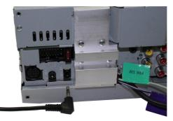
4. Select the correct harness (8-way ISO or Quadlock) for your vehicle. Connect the 14 way molex connector to the interface
