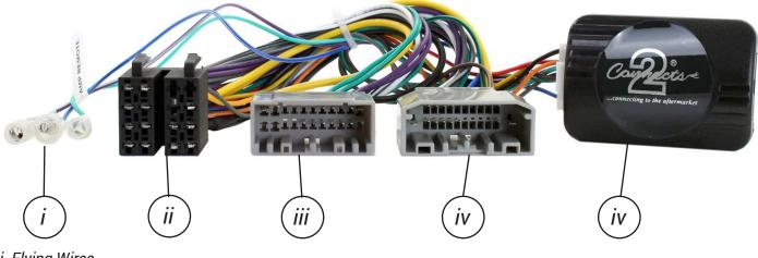
i. Flying Wires ii. ISO Connector (16 Pin) iii. OEM Connector Variant 1 (22 Pin) iv. OEM Connector Variant 2 (22 Pin) v. Interface Box
