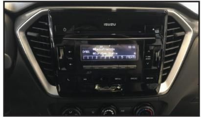
Note: this installation kit will work with both OEM single DIN and touch screen system layouts.
