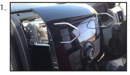
Use a set of release keys to pry the head unit out of the dashboard. Dependent on the style of unit you have installed, you will need either single or double DIN keys. Once released, take out the unit and disconnect all the wiring.
