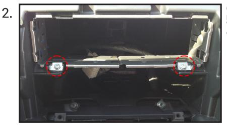
Once the main head unit is out of the way, proceed to remove the highlighted screws. When done, proceed to fully remove the cage.
