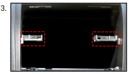
The highlighted area(s) on the inner dash will need to be cut out in order to allow the new double DIN unit to sit correctly.
