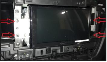
With the brackets attached and the connections made to the rear of the radio, place the unit into the dashboard and screw into place using the four pre-exisiting screws removed in earlier (see Step 2).
