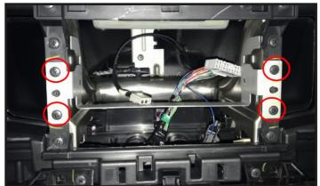
With the main fascia panel out of the way, undo the following four screws and put these to one side. With the screws out, fully remove the metal bracket.
