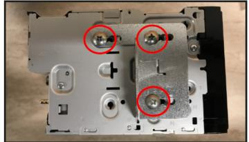
Take the brackets found within the kit and offer them up to the relevant side of the new radio. Once positioned correctly, screw them into place using a set of radio screws (not supplied with this kit).
