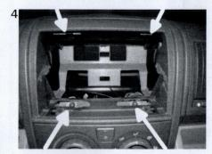
4 Remove the four screws as shown.
