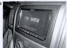
9 Connect all cables, mount the aftermarket car-radio + brackets to the brackets previously fitted inside the housing using the four screw supplied.
