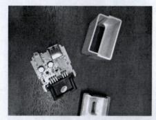
Open the front plastic cover and remove the original PCB. Save the white plastic after removing the PCB.
