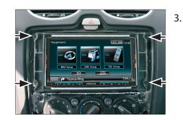
. Push the head unit with the mounted metal brackets into the metal frame, until it snaps in
