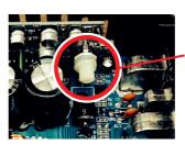
About potentiometer (red circle) the sensitivity of the signal detection can be adjusted continuously.
